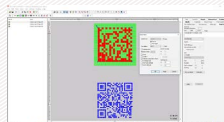
Reading & grading of several 2D codes (QR-Code, Datamatrix) in a large marking window (170 x 170). Reading possible in the entire marking window.
