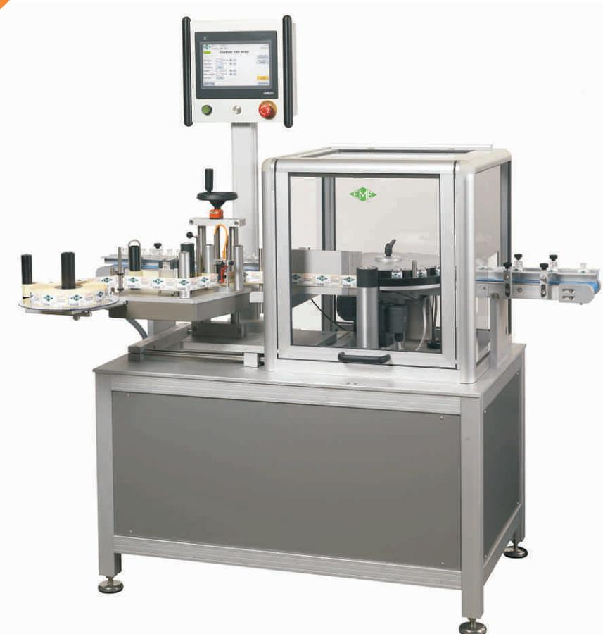
The star wheel construction in this system, provides a high capacity and a high quality in labelling.
