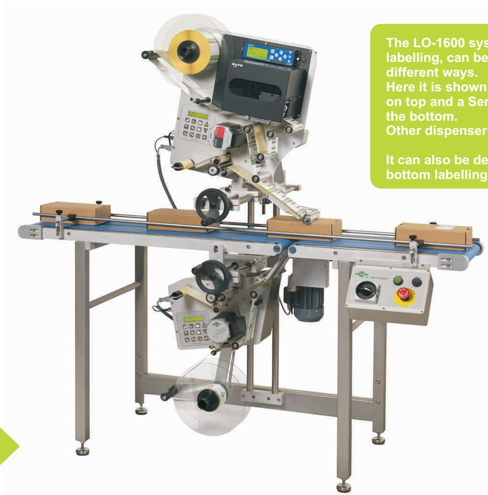
The LO-1600 system for top-bottom labelling, can be configured in different ways. Here it is shown with a Series 3000 on top and a Series 2000 at the bottom. Other dispenser models can be used.
