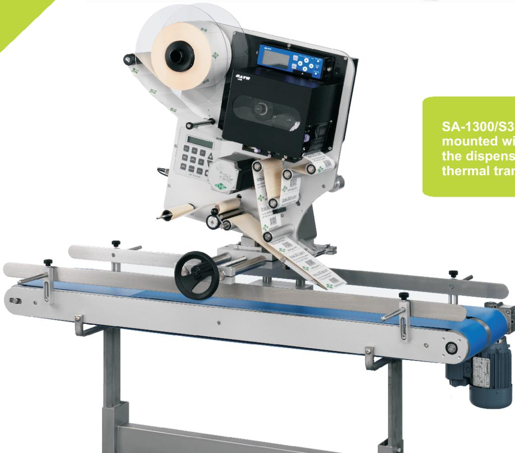
SA-1300/S3 - top labelling system mounted with EME Series 3000, the dispenser combined with a thermal transfer printer.
