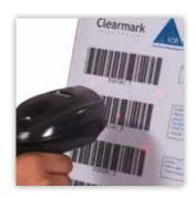
USB scanpoint feature allows job selection via barcode scanning with no operator intervention and no human error.
