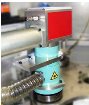
Protective sleeve for laser
