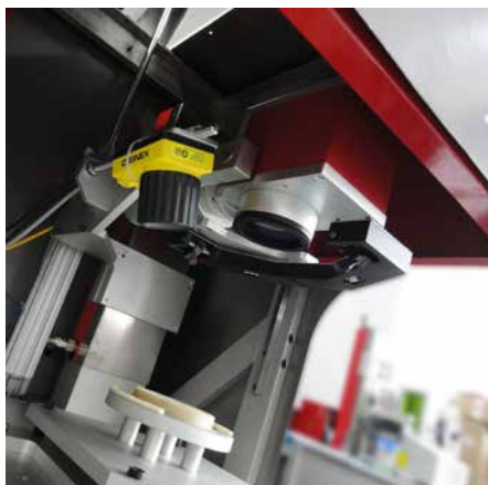
XL-Box marking station with deported reading system
