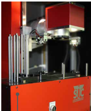
Loading area for blank plates
